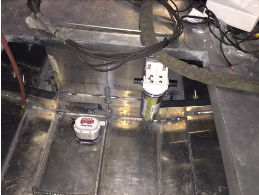
Miscellaneous Outfitting Tasks (Battery/Bilge/fuel filter)
