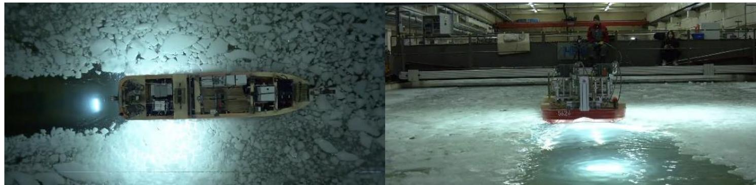
Ice Management Astern in the HSVA Test Basin (30° toe-in angle)
