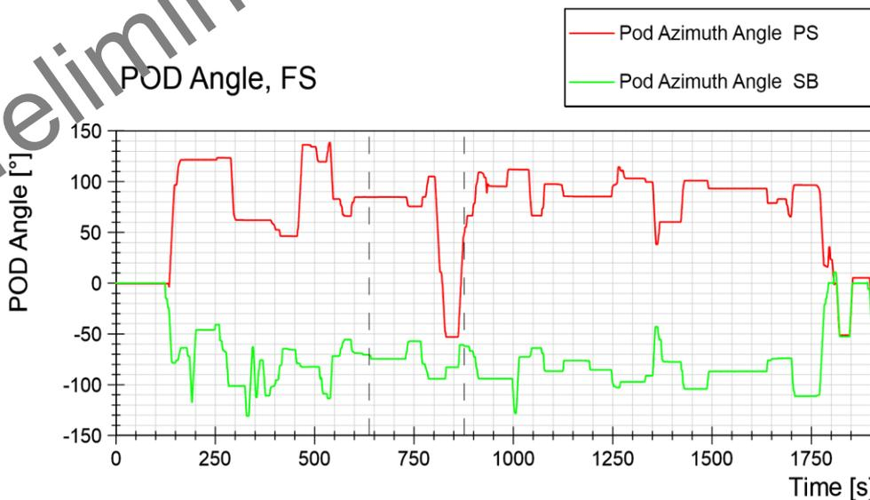
*Figure 155 Test run no. 35010R, free running test ahead, POD angle*
