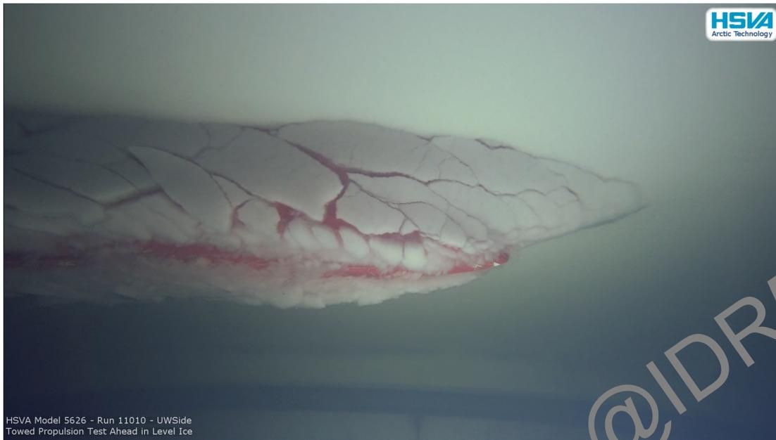
**Figure 11: Icebreaking Astern in 1.37m Ice Thickness**
