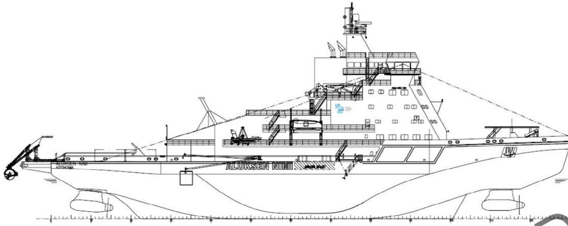
**Figure 3 – PC4 Icebreaking Vessels Polaris with bow azipod**
