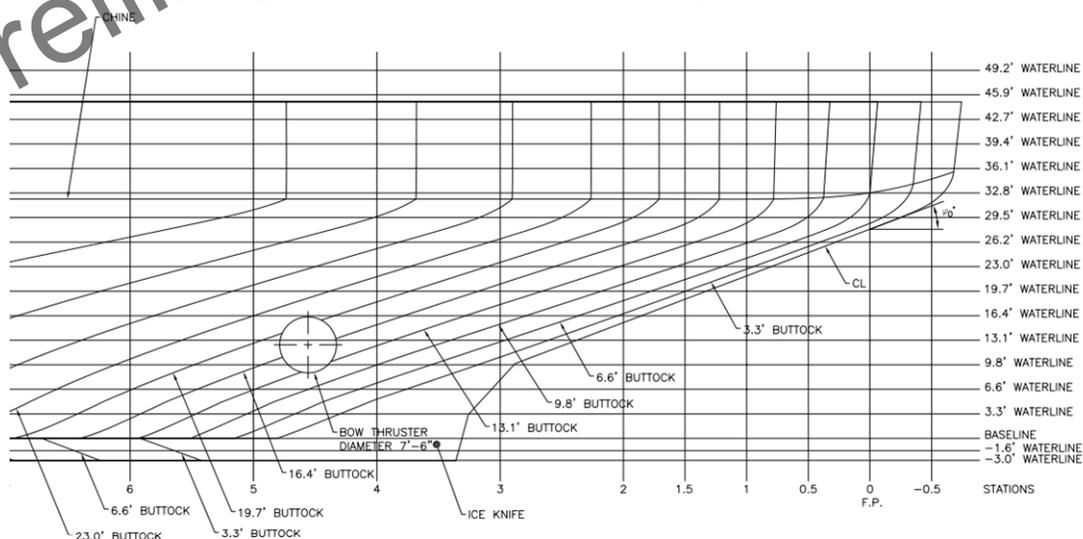
**Figure 1 – Baseline Tunnel Thruster Illustration**
