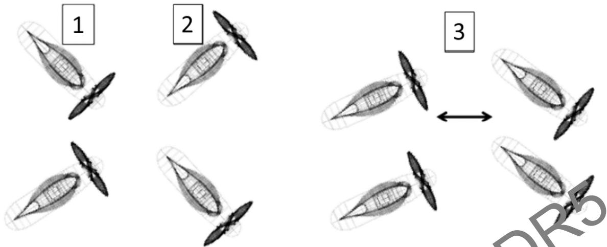
Figure 21: Clear Channel in 3.3 ft of Unbroken Ice
