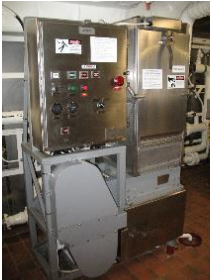
Figure 7 Commercial-scale metal/glass shredder
