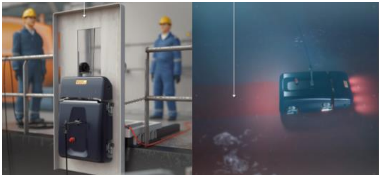
Figure 1 Jotun HullSkater robotic inspection and cleaning ROV
