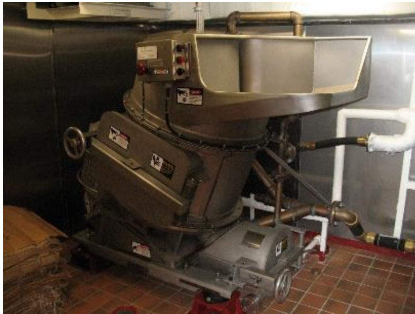
Figure 5 Example of a commercial scale pulper for processing shipboard food, cardboard, and paper.
